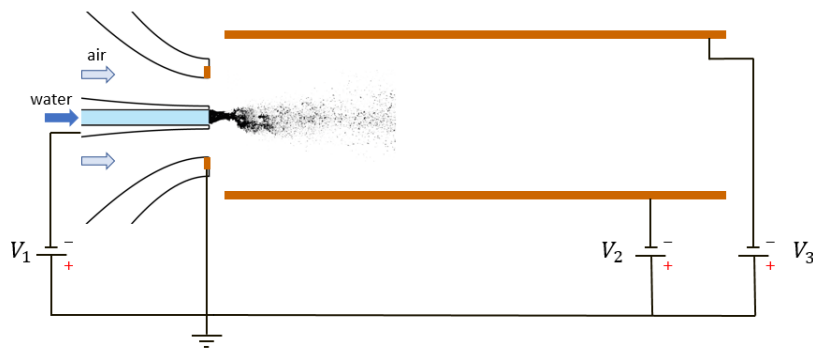
Figure 1. Schematics of the canonical coaxial two-fluid atomizer. The potential V_1 is set at -5 kV to charge the liquid, while the plate configuration can be V_2 = V_3 = 0 for outward electric forcing, V_2 = V_3 = -5 kV for an inward electric forcing and V_2 = -5 kV and V_3 = 0 for an upward electric forcing.
