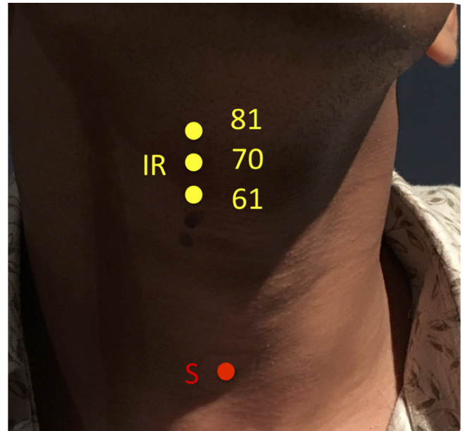
Fig. 2. Illustration of ePGG fixed subglottal light sensor (S) position and 3 supraglottal source (IR) positions along the front neck surface and source-sensor distances d [mm].
